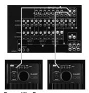
Preamplifier Processor (Unbalanced RCA to Unbalanced RCA)
